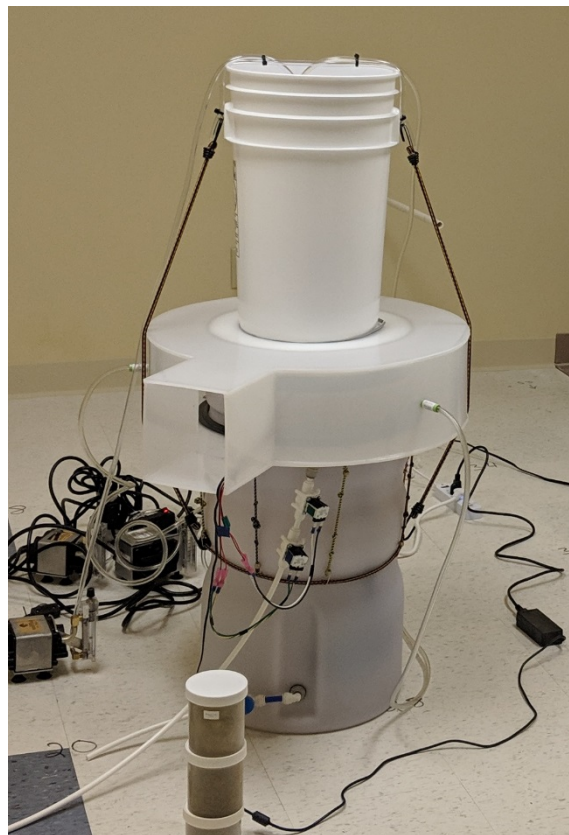
Figure 2. Air Recirculation attachment mounted on an CAZ-100B System for experimental trials. System is completely sealed off from external air during trials. Sampling ports on the sides, top and back allow for measuring spore concentrations.
